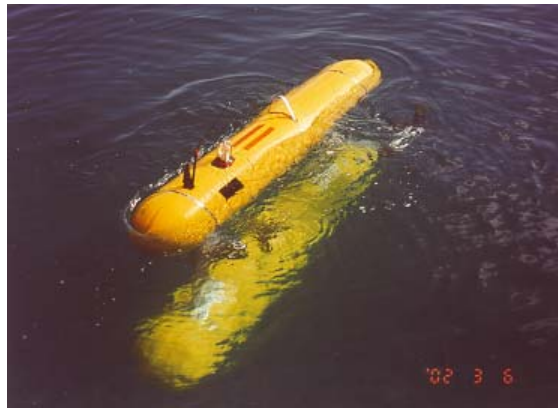
Figure 11. The Seabed - a hover capable AUV developed by Hanu Singh at WHOI
